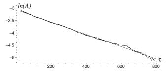
Fig. 4. The amplitude  $A(\tau)$  on the logarithmic scale: experimental curve (bold) and a linear fit (thin). The same run as the one shown in Figs. 1, 2 and 3.
