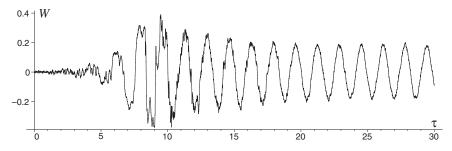
Fig. 2. The piston velocity W as a function of time  $\tau$ . The same run as in Fig. 1.
