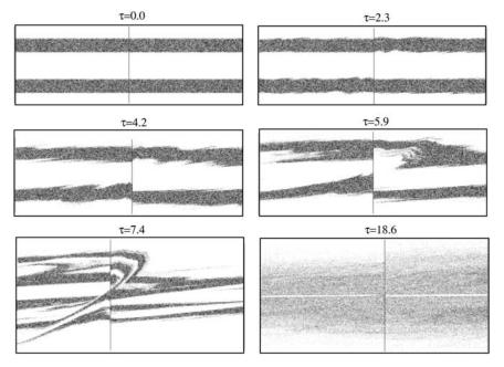
Fig. 6. Six snapshots of the empirical gas density (in the x, v plane) at times  $\tau = 0$ , 2.3, 4.2, 5.9, 7.4 and 18.6.
